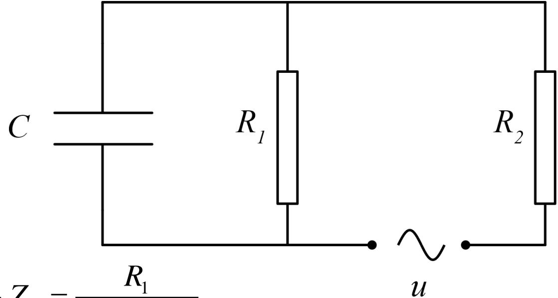
$$\frac{1}{Z_p} = \frac{1}{R_1} + \frac{1}{-j \cdot \frac{1}{\omega C}} = \frac{1}{R_1} + j\omega C = \frac{1 + j\omega CR_1}{R_1} \Rightarrow Z_p = \frac{R_1}{1 + j\omega CR_1}$$
